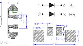
Tolerance: ±0.10mm Recommend Soldering Pattern unless otherwise note(Units:mm)
